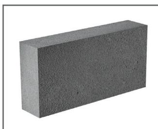
**Aircrete blocks** – These are lighter than aggregate blocks, as they are made from a type of concrete that contains millions of tiny air bubbles trapped within the block. No aggregates larger than ground sand are used. The presence of air bubbles reduces the block density, which can aid manual handling and provides an increase to the overall insulation properties of the wall.
